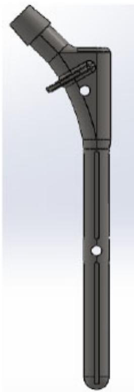
**Figure 1.** UNDIP femoral stem design.
